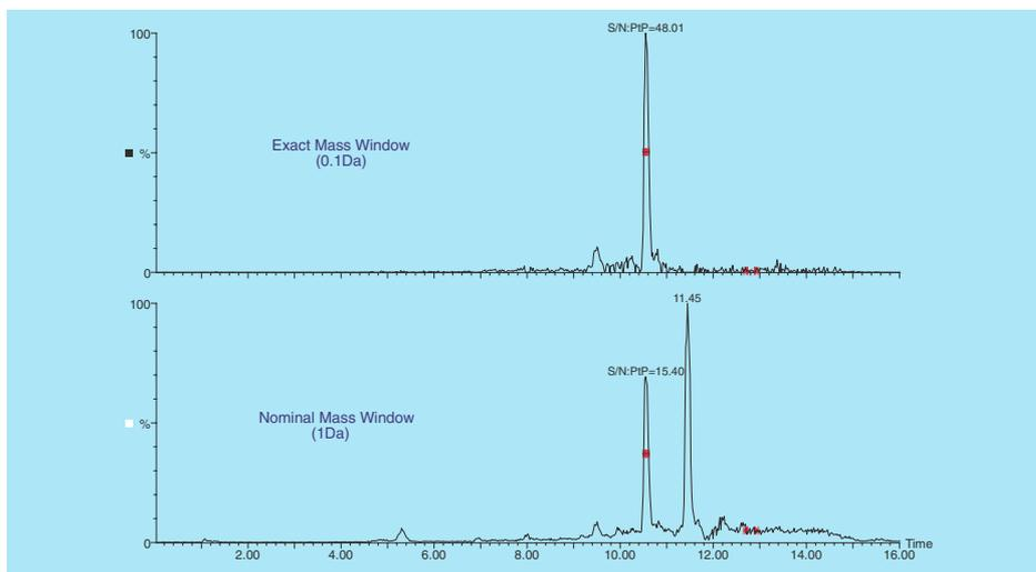
Figure 5. Signal to Noise Comparison of Exact and Nominal Mass Chromatograms.
