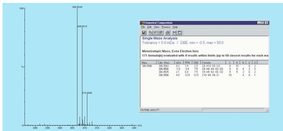
Figure 8. Exact Mass Spectrum of Unknown Pesticide (Buzzard Sample).
