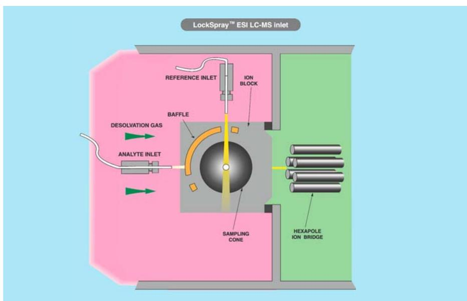
Figure 2. Dual Electrospray Schematic.
