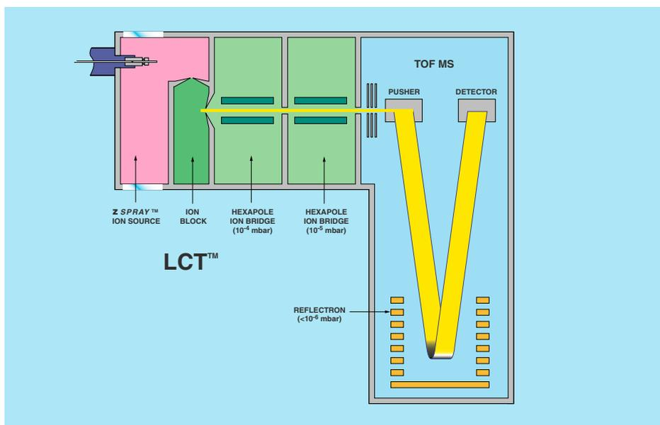
Figure 1. Schematic Diagram of Micromass LCT.
