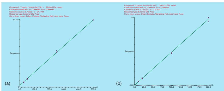
Figure 6a and 6b. Quantitation Calibration Graphs for Carbosulfan and Fenarimol.
